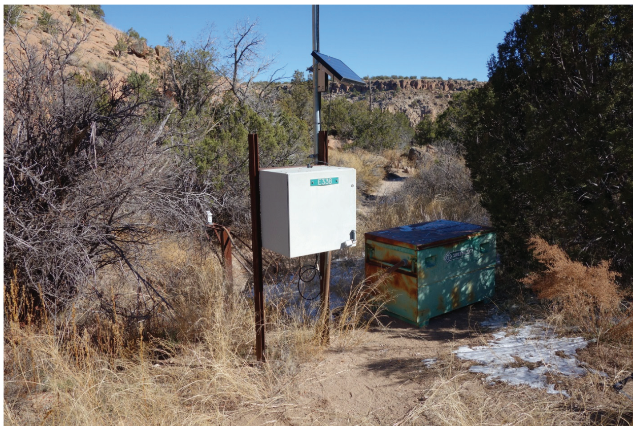
E338 Stream gaging station, downstream view
