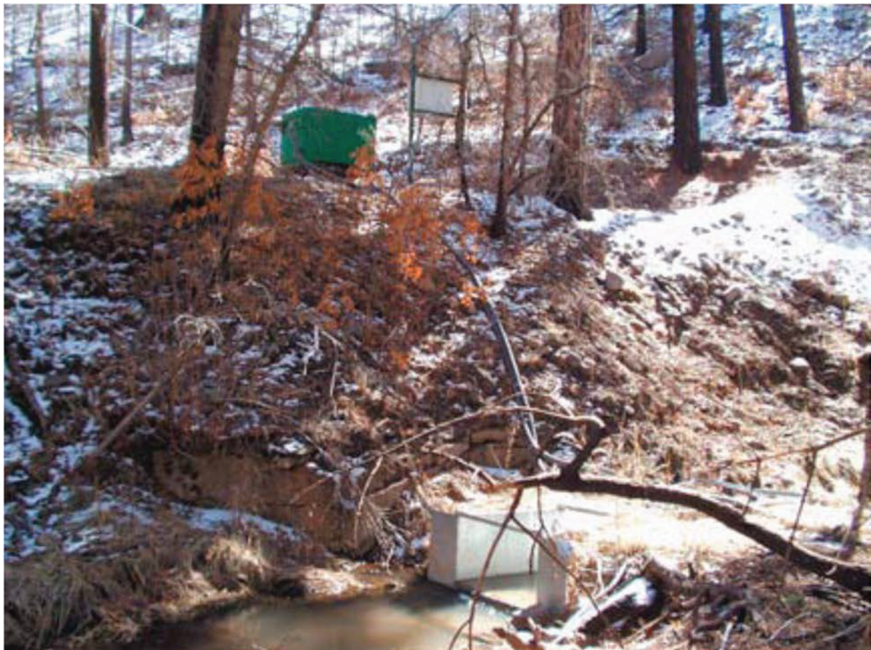
E256 Stream gaging station, upstream view
