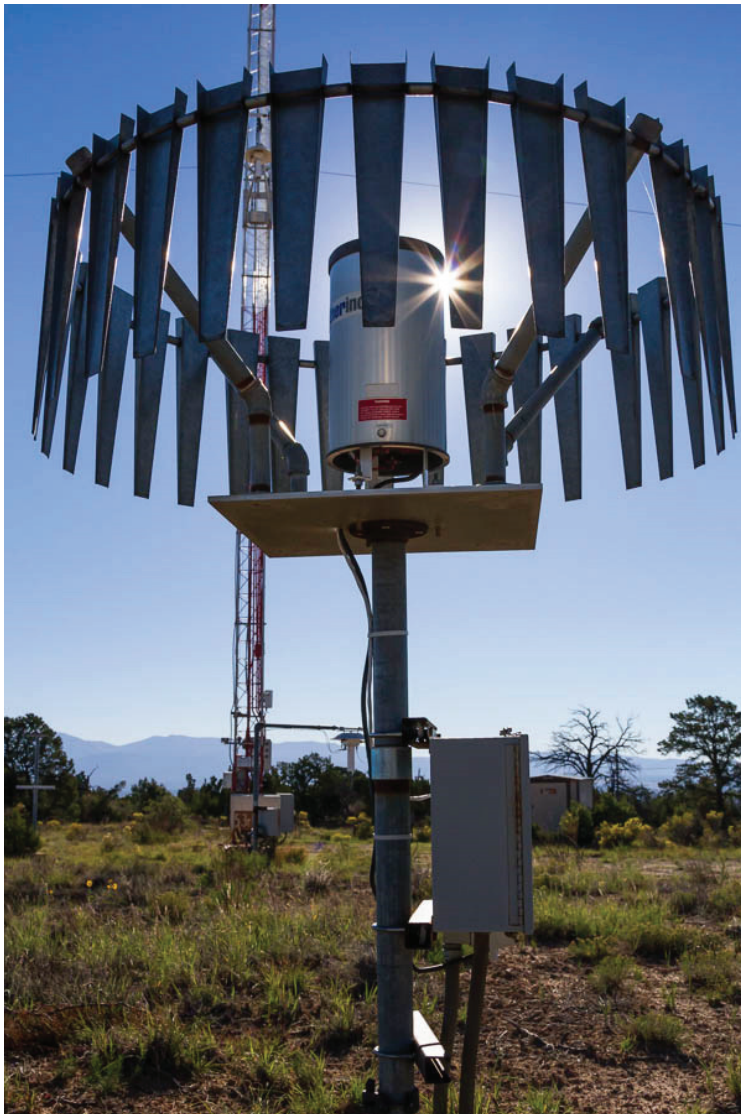
RG-TA-53 Precipitation gaging station (foreground) and meteorological tower (background)
