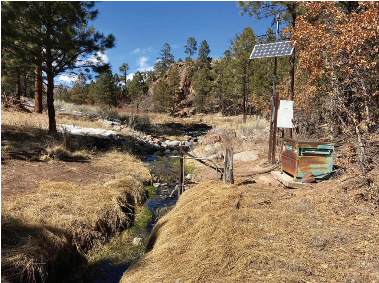
E123 Stream gaging station, upstream view
