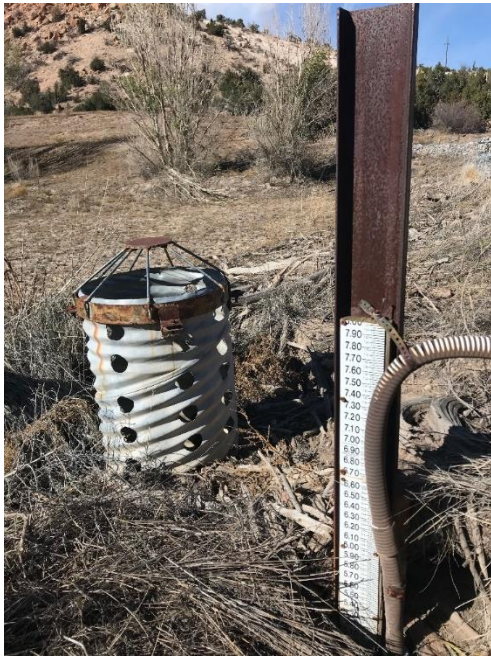
Photo C-4.4-2 October 2021—Standpipe. Debris is at staff plate height 5.4 ft and sediment is at 4.8 ft; this correlates to 61% of storage capacity remaining. No significant change since last inspection.
