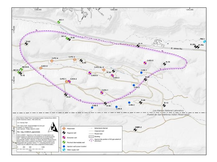
Figure 1. Map showing the locations of pumping well CrEX-1, injection wells CrIN-1 and CrIN-2, and other locations at which monitoring will take place
