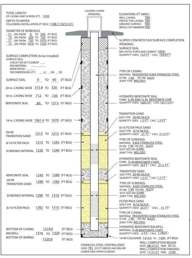
Well R-72 As-Built Well Construction Diagram
