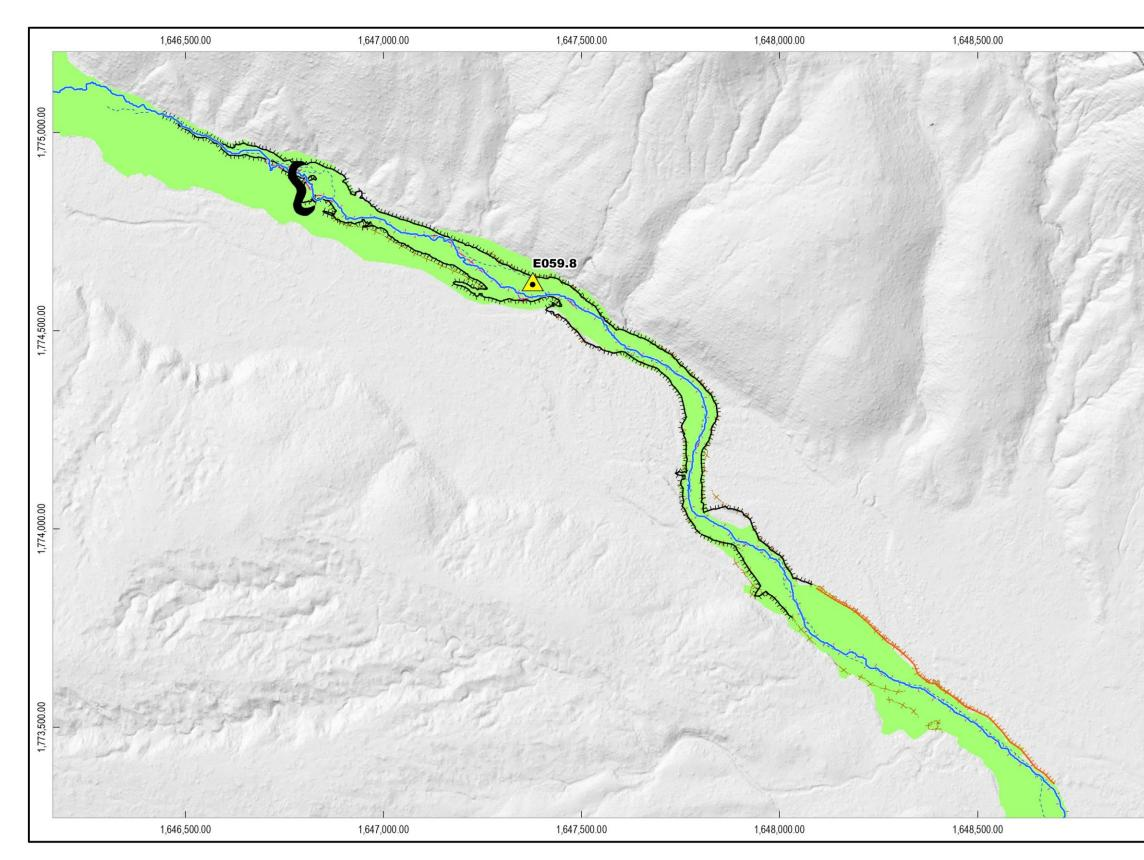
Figure B-4.1-2 Comparison of thalweg and banktop surveys near gage station E059.8
