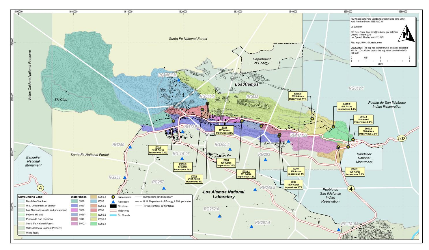
Figure 2.1-4 LA/P watershed showing drainage areas for each stream gaging station and associated rain gages and Thiessen polygons
