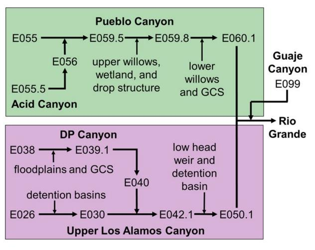
Figure 3.2-1 Flow diagram of gaging station the LA/P watershed
