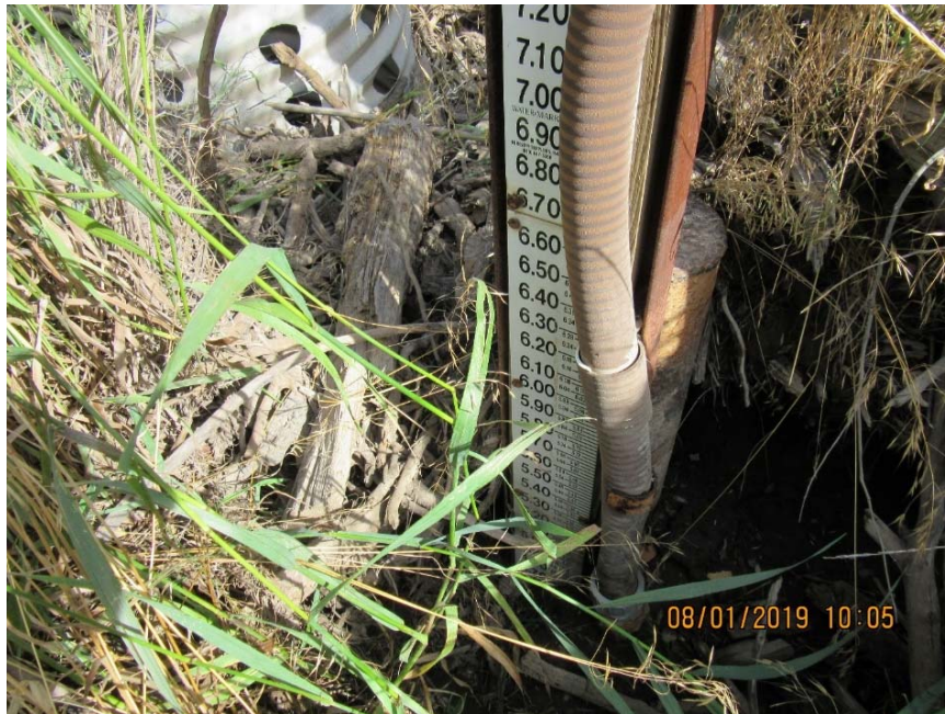
Photo C-4.9-2 Flow event inspection for July 26, 2019, storm event—standpipe. Sediment is approximately 4 ft deep. Debris accumulation (branches, pinecones, plastic bottles) is approximately 2 ft above sediment level. Approximately 3 ft of standpipe exposed.
