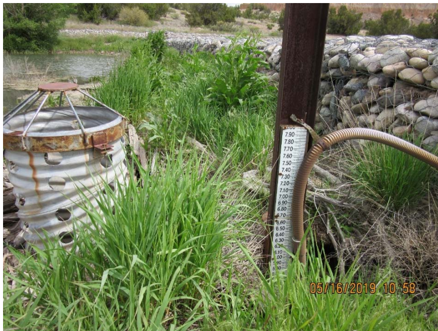
Photo C-4.9-1 May 2019—standpipe. Gage reads approximately 6 ft of sediment and debris. Approximately 3 ft of standpipe exposed. No deficiency found.
