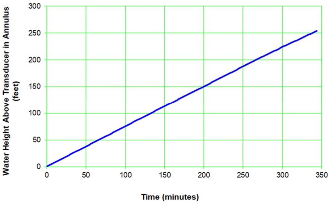
Figure C-11.3-1 Well R-19 screen 2 initial refill response
