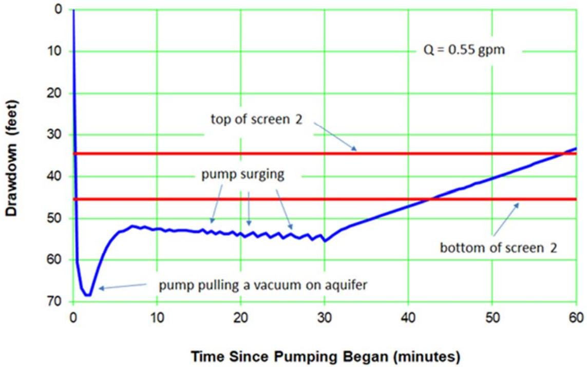
Figure A-5.0-3 Well R-9i screen 2 initial pumping test response
