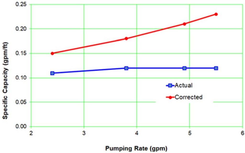
Figure A-4.0-2 Well R-8 screen 1 actual and corrected specific capacities
