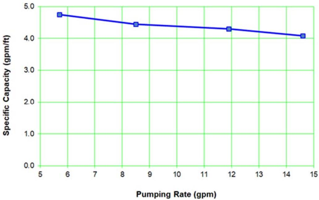
Figure A-5.0-2 Well R-9i screen 1 specific capacities
