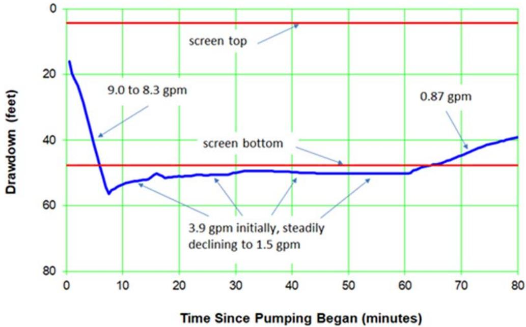
Figure A-2.0-2 Well R-5 screen 3 initial pumping test response
