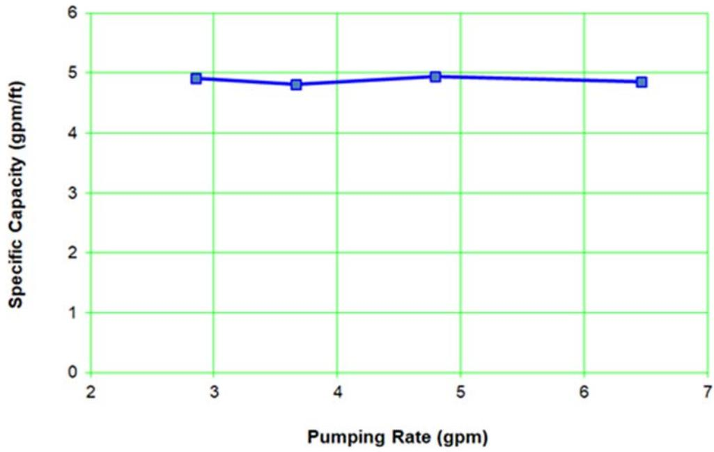
Figure A-6.1-2 Well R-19 screen 3 specific capacities after jetting
