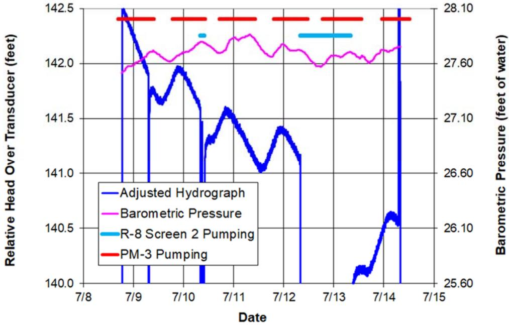
Figure C-9.2-3 Well R-8 screen 2 adjusted hydrograph during screen 2 pumping test
