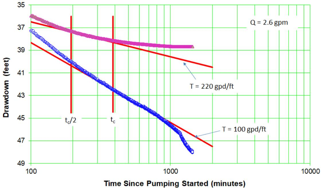
Figure C-7.3-2 Well R-5 screen 2 drawdown – expanded scale
