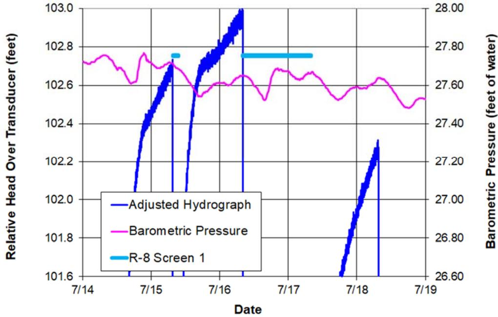
Figure C-9.2-1 Well R-8 screen 1 adjusted hydrograph during screen 1 pumping test
