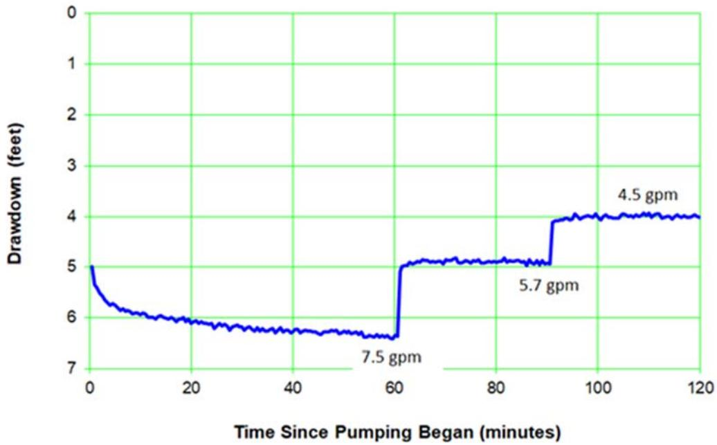
Figure A-4.0-3 Well R-8 screen 2 initial step-drawdown test response
