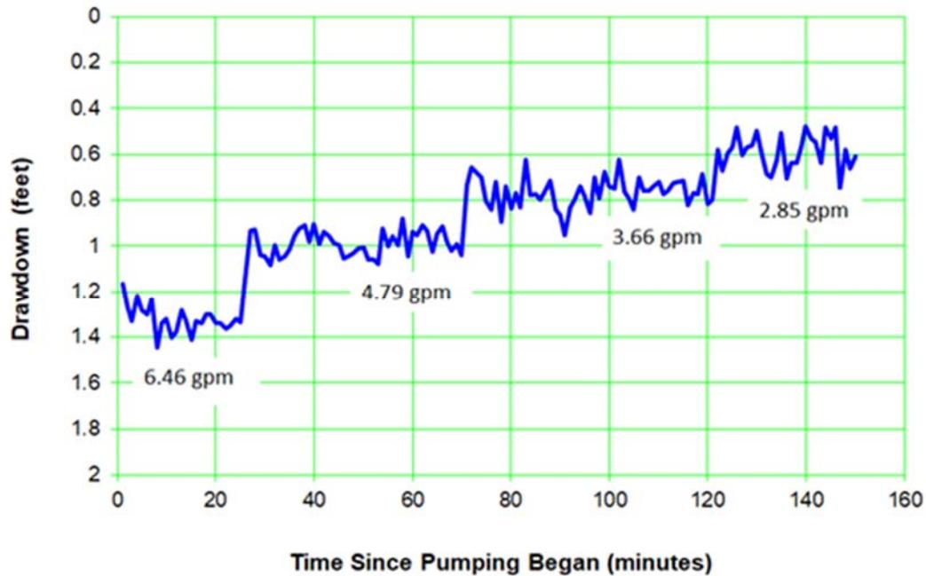
Figure A-6.1-1 Well R-19 screen 3 step drawdown test response after jetting
