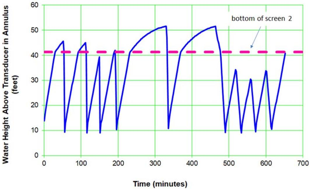
Figure C-11.3-5 Well R-19 screen 2 pumping and refill response
