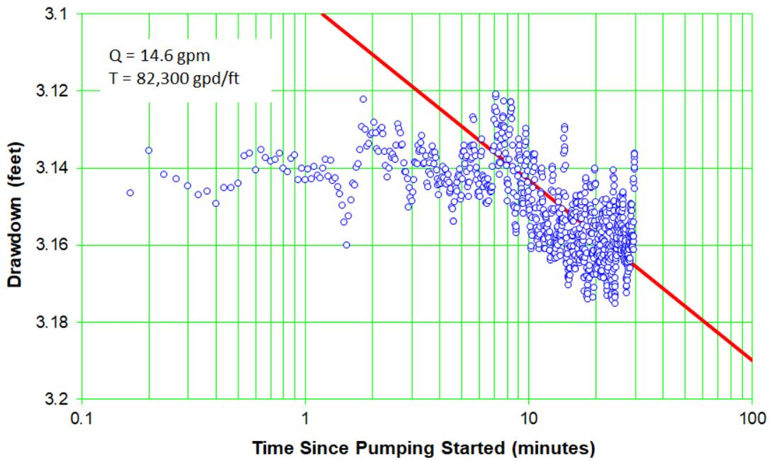
Figure C-10.3-2 Well R-9i screen 1 trial 1 rolling average drawdown – expanded scale
