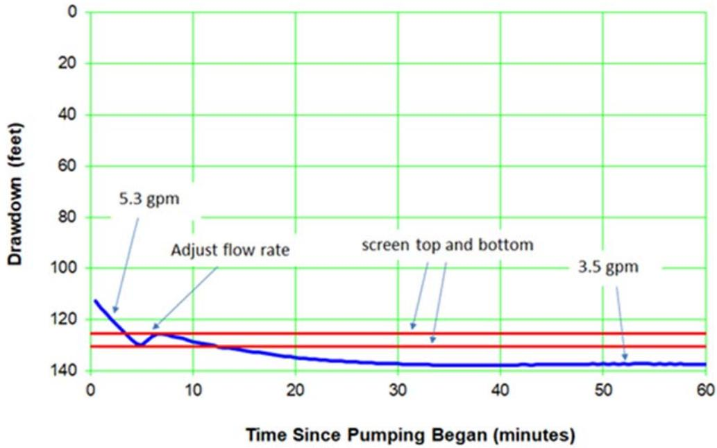
Figure A-2.0-3 Well R-5 screen 4 initial pumping test response
