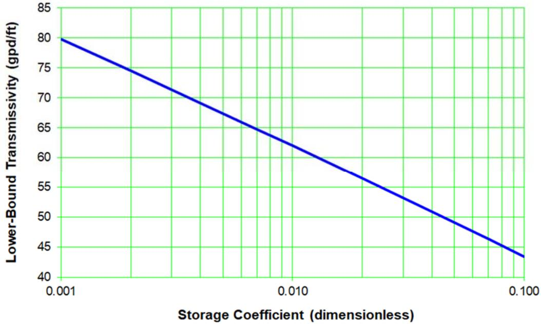
Figure C-7.4-1 Well R-5 screen 2 lower-bound transmissivity
