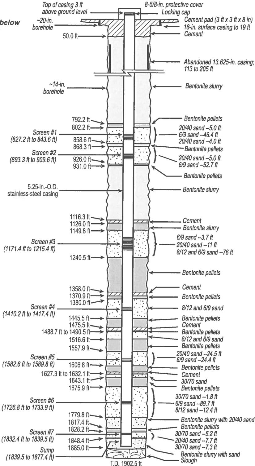
Note: The screen intervals list the footages of the pipe perforations, not the tops and bottoms of screen joints.
