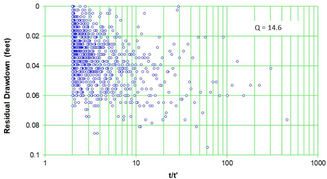
Figure C-10.3-4 Well R-9i screen 1 trial 1 recovery – expanded scale
