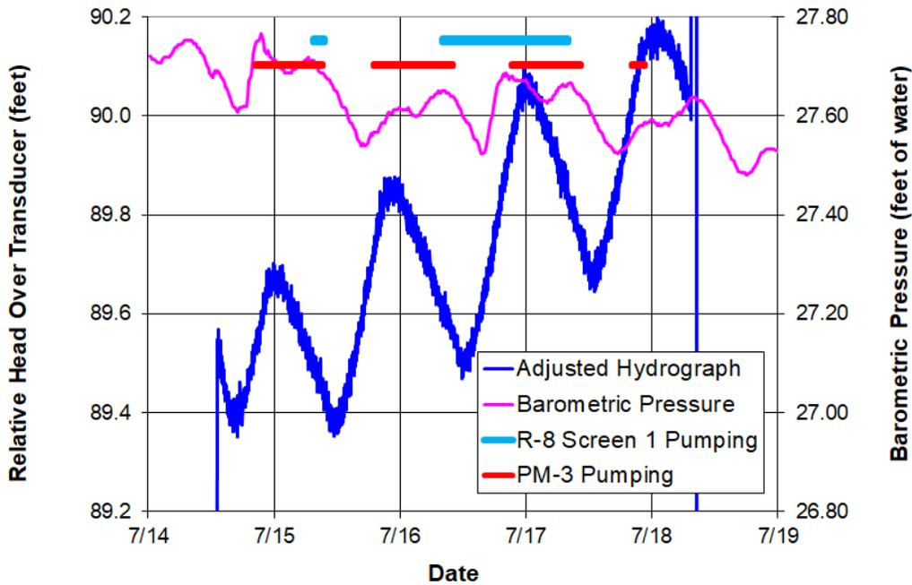
Figure C-9.2-2 Well R-8 screen 2 adjusted hydrograph during screen 1 pumping test
