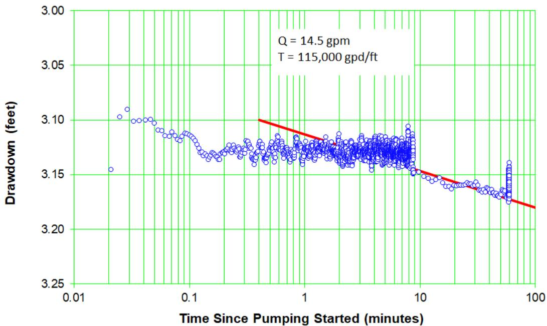
Figure C-10.3-8 Well R-9i screen 1 trial 2 drawdown – expanded scale
