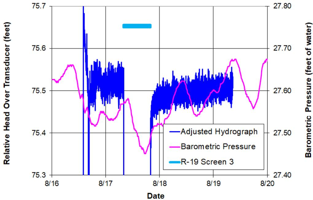
Figure C-11.2-3 Well R-19 screen 3 adjusted hydrograph
