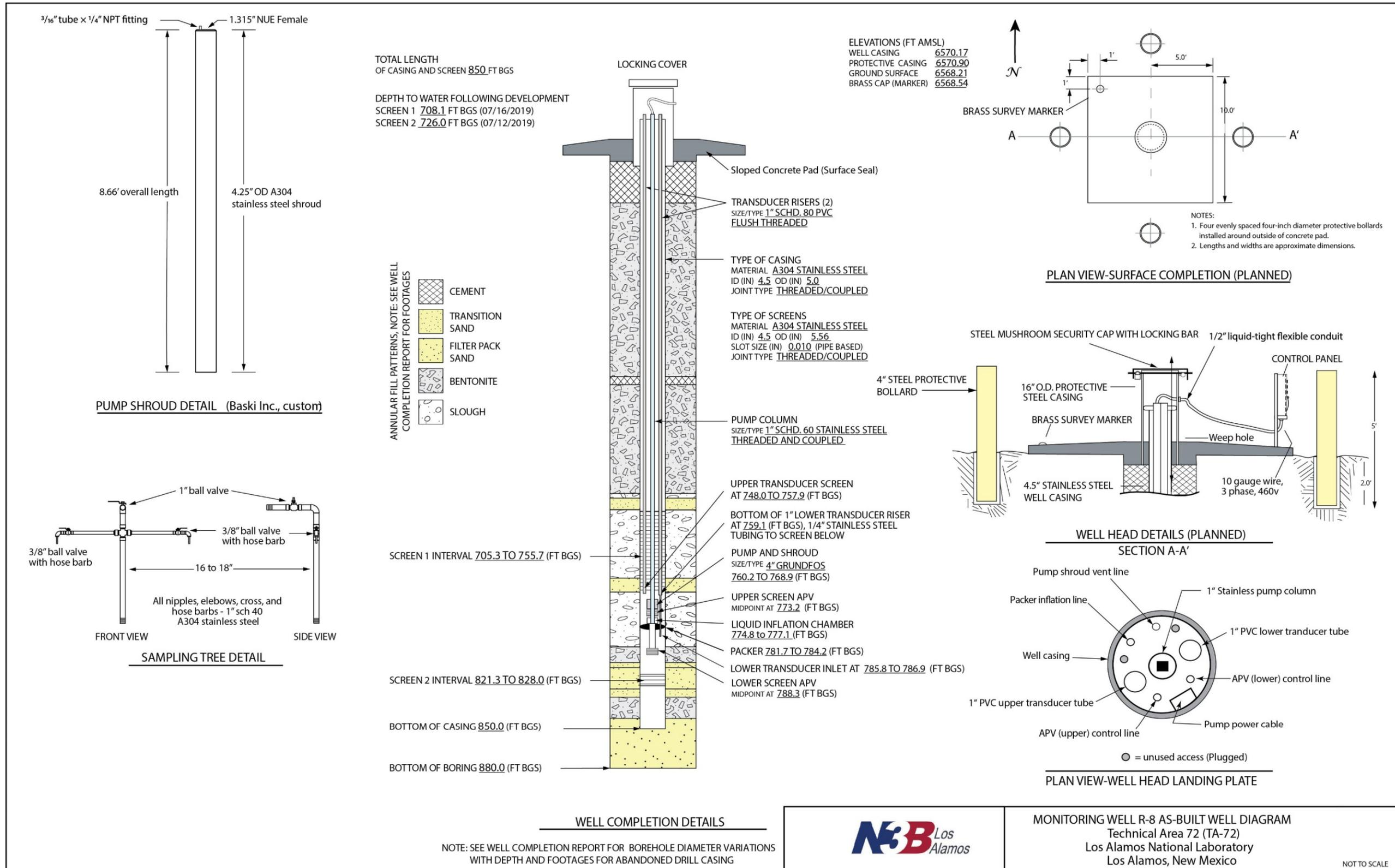
Figure 2.3-1 Monitoring well R-8 as-built construction diagram post-Westbay conversion
