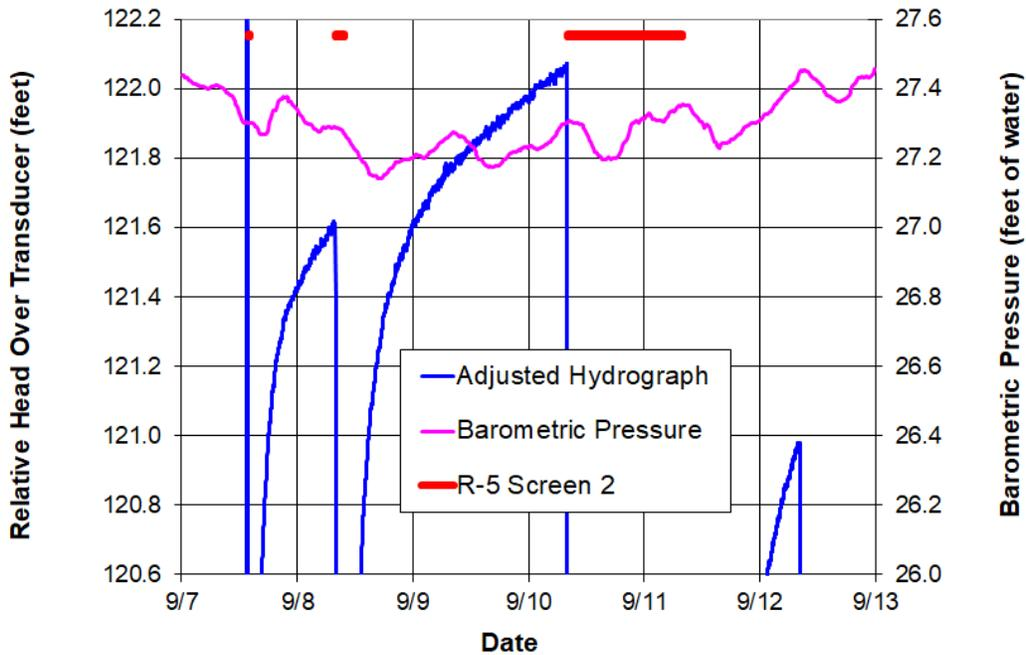
Figure C-7.2-2 Well R-5 screen 2 adjusted hydrograph – rolling average
