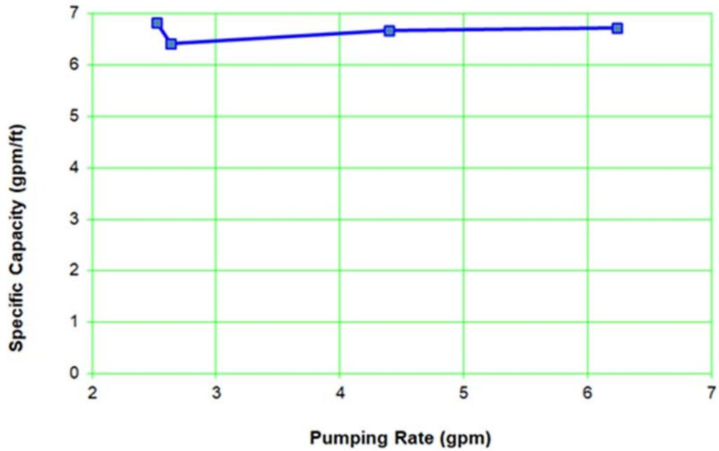
Figure A-6.0-2 Well R-19 screen 3 specific capacities (screens 3 through 7 open)
