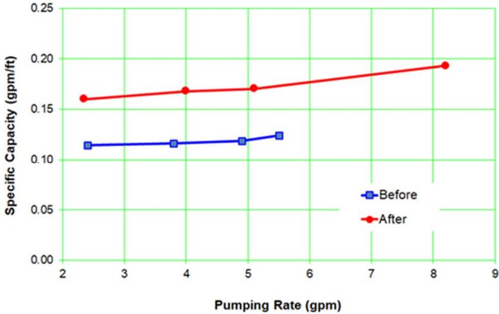
Figure A-4.1-2 Well R-8 screen 1 specific capacities before and after jetting
