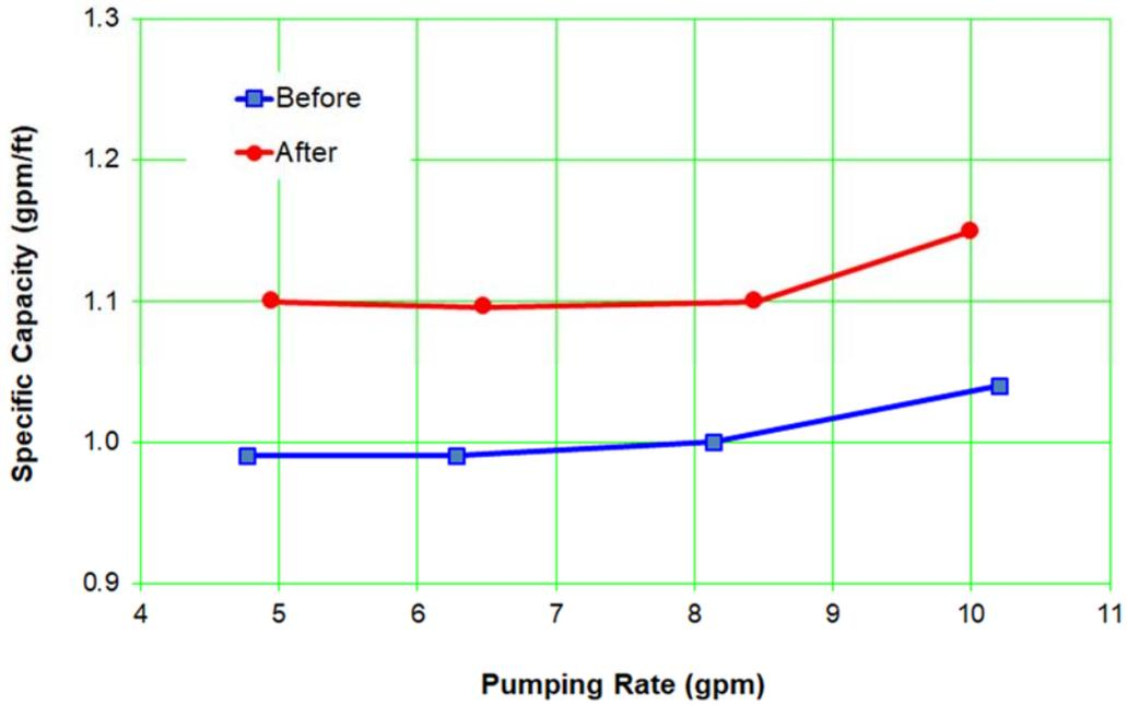
Figure A-3.1-2 Well R-7 screen 3 specific capacities before and after jetting
