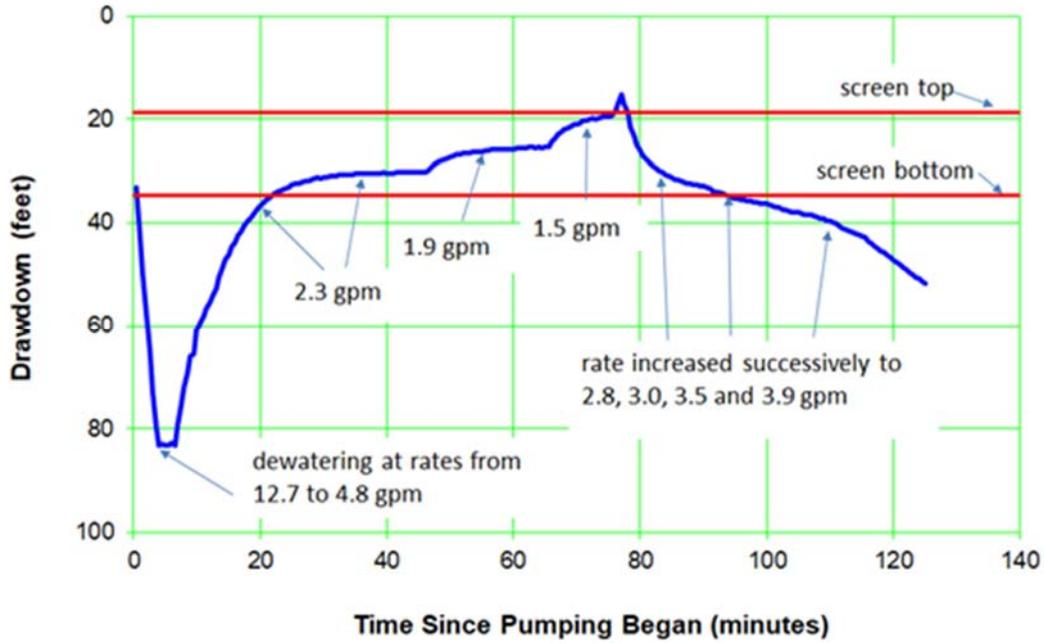
Figure A-2.0-1 Well R-5 screen 2 initial pumping test response
