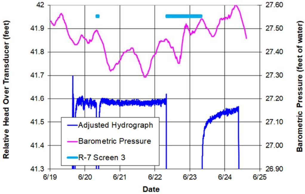
Figure C-8.2-2 Well R-7 screen 3 adjusted hydrograph – rolling average
