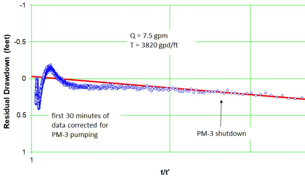
Figure C-9.5-5 Well R-8 screen 2 trial 2 recovery – expanded scale
