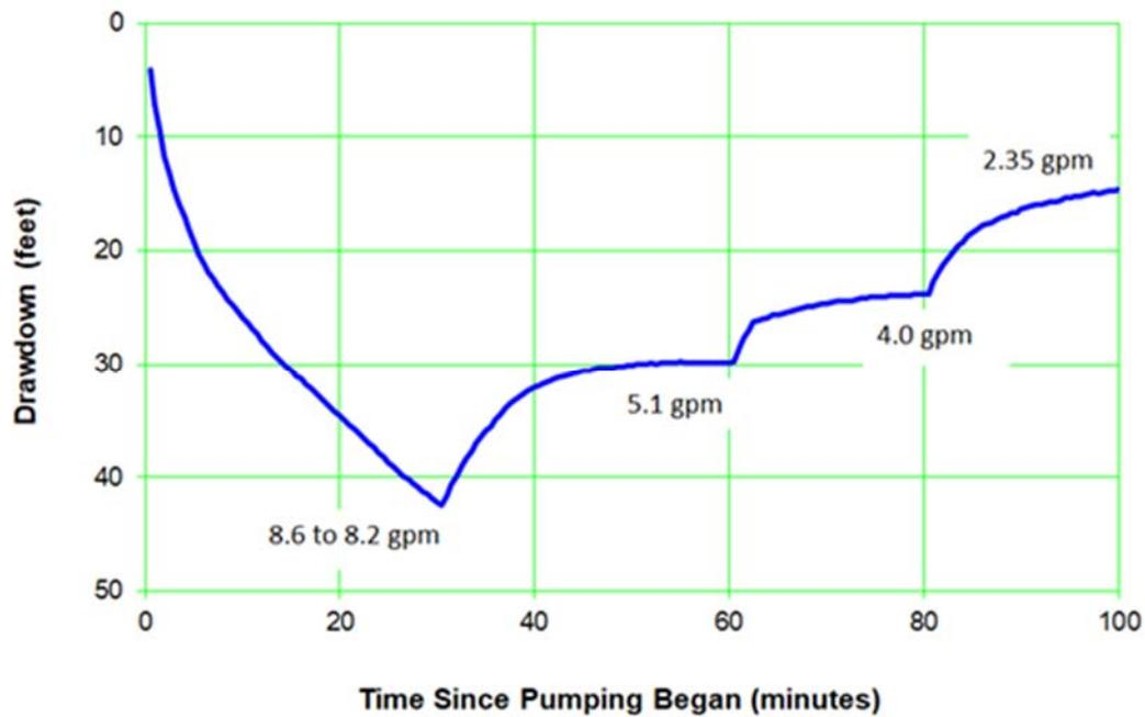
Figure A-4.1-1 Well R-8 screen 1 step-drawdown test response after jetting
