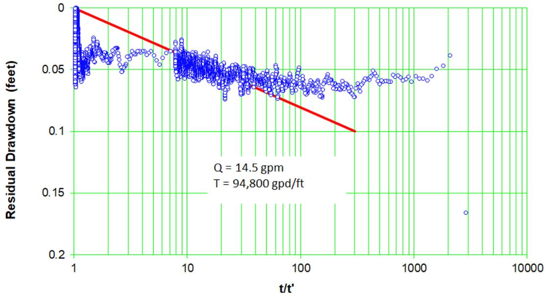
Figure C-10.3-11 Well R-9i screen 1 trial 2 recovery – rolling average
