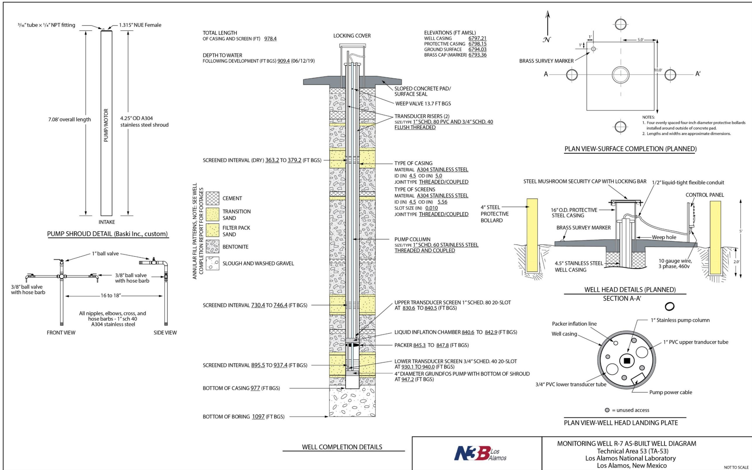
Figure 2.2-1 Monitoring well R-7 as-built construction diagram post-Westbay conversion
