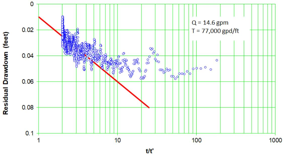
Figure C-10.3-5 Well R-9i screen 1 trial 1 recovery – rolling average
