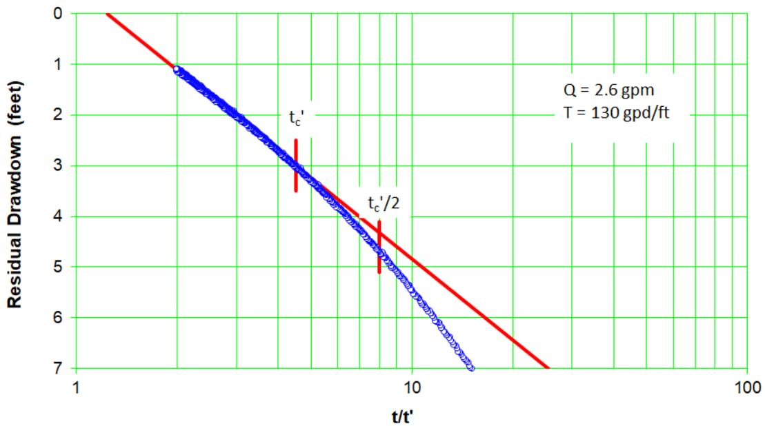
Figure C-7.3-4 Well R-5 screen 2 recovery – expanded scale
