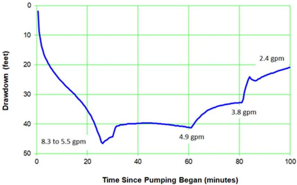
Figure A-4.0-1 Well R-8 screen 1 initial step-drawdown test response
