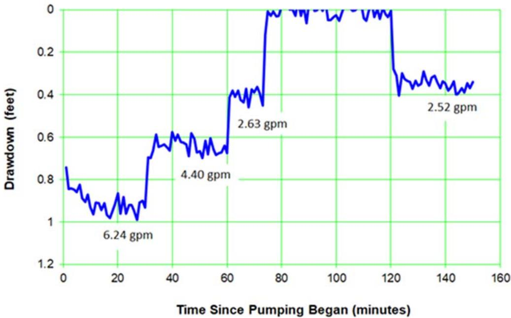
Figure A-6.0-1 Well R-19 screen 3 initial step-drawdown test response (screens 3 through 7 open)
