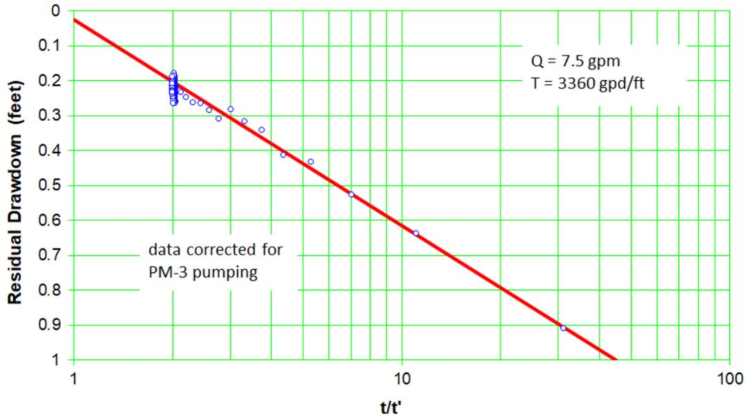
Figure C-9.5-2 Well R-8 screen 2 trial 1 recovery
