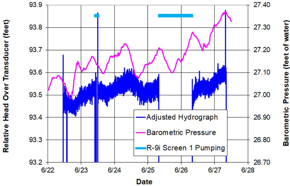
Figure C-10.2-1 Well R-9i screen 1 adjusted hydrograph
