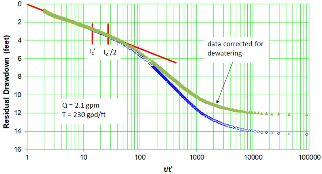
Figure C-9.3-3 Well R-8 screen 1 recovery corrected for dewatering
