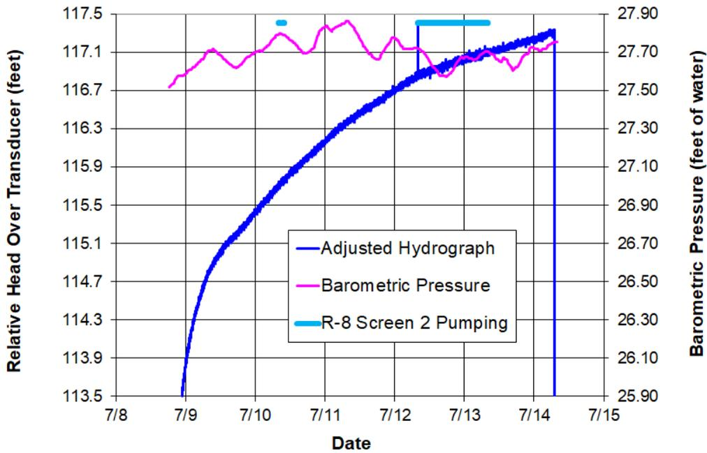
Figure C-9.2-4 Well R-8 screen 1 adjusted hydrograph during screen 2 pumping test
