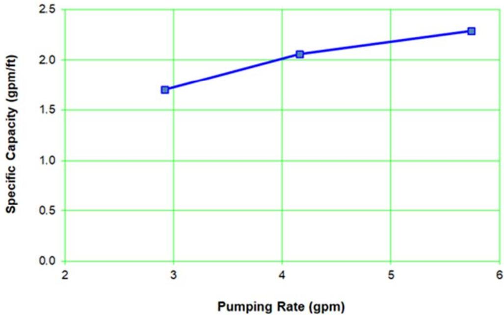
Figure A-6.0-4 Well R-19 screen 4 specific capacities
