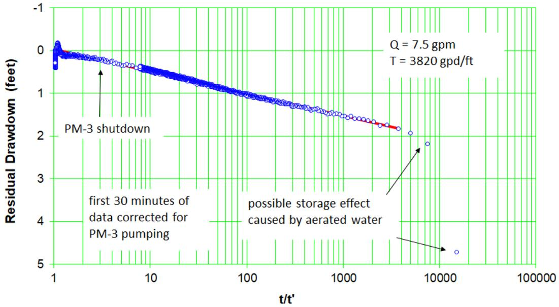
Figure C-9.5-4 Well R-8 screen 2 trial 2 recovery
