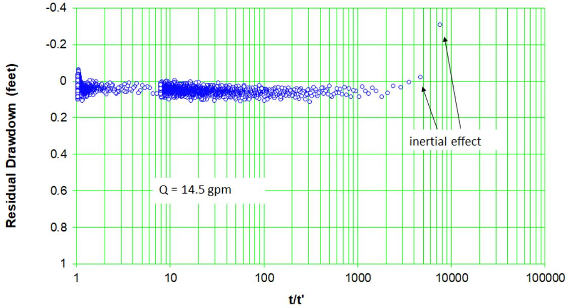
Figure C-10.3-9 Well R-9i screen 1 trial 2 recovery
