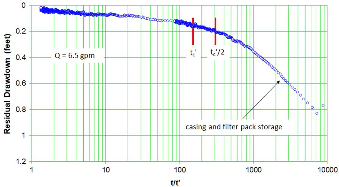
Figure C-11.5-4 Well R-19 screen 3 recovery – rolling average
