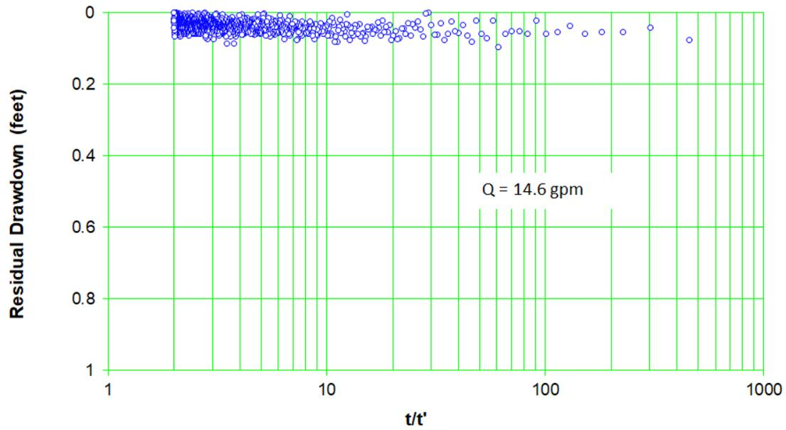
Figure C-10.3-3 Well R-9i screen 1 trial 1 recovery
