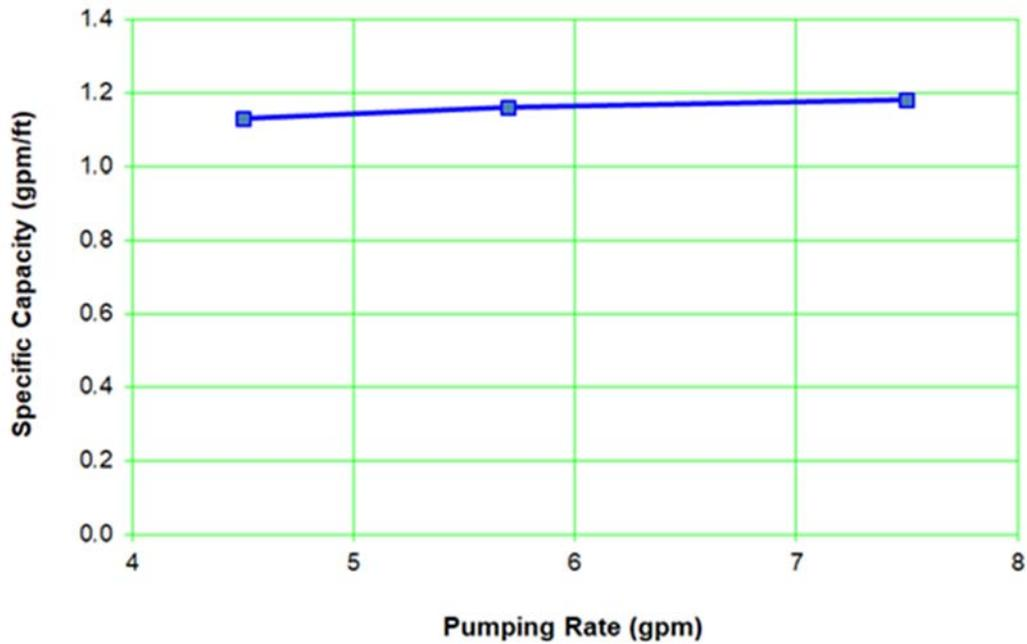
Figure A-4.0-4 Well R-8 screen 2 specific capacities
