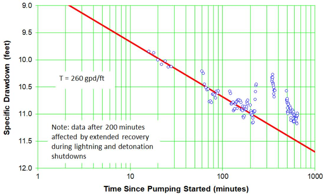
Figure C-11.3-9 Well R-19 screen 2 specific drawdown – extended test
