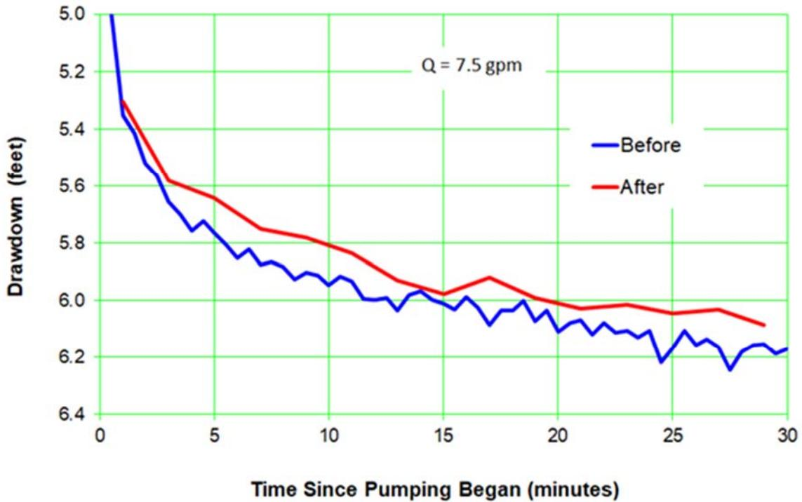
Figure A-4.1-3 Well R-8 screen 2 drawdown before and after jetting
