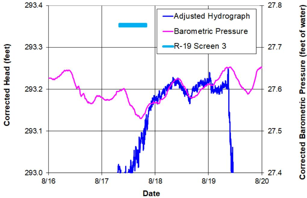
Figure C-11.2-2 Well R-19 screen 2 corrected for 0.105 ft/day water level rise and 55% barometric efficiency
