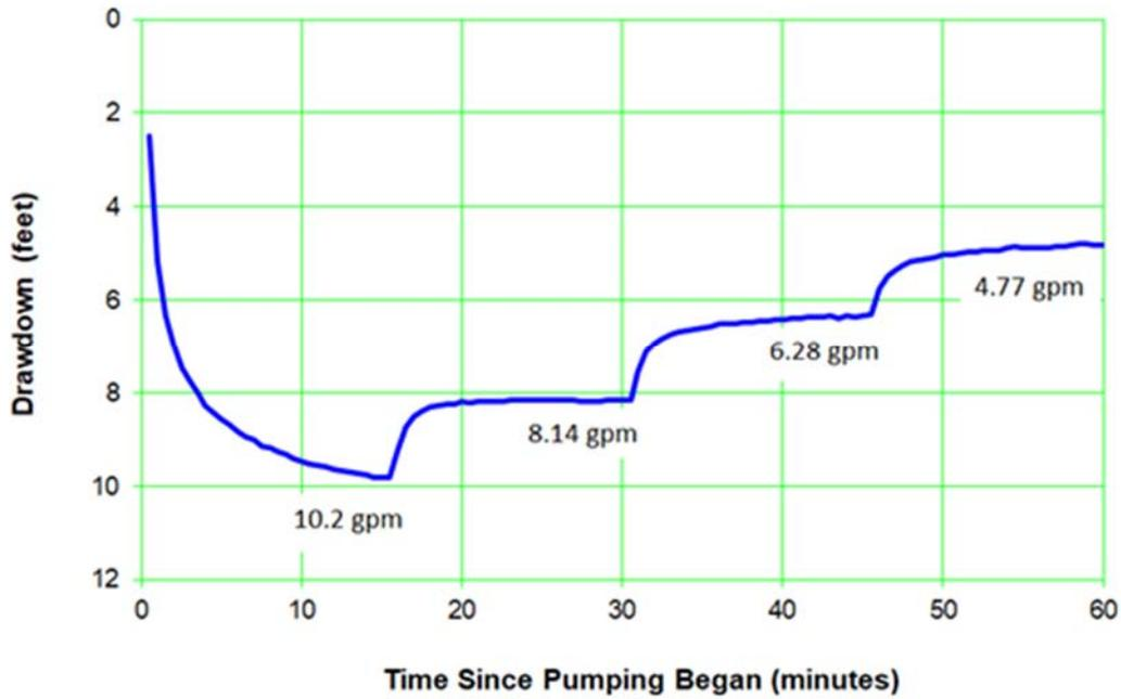
Figure A-3.0-1 Well R-7 screen 3 initial step-drawdown test response
