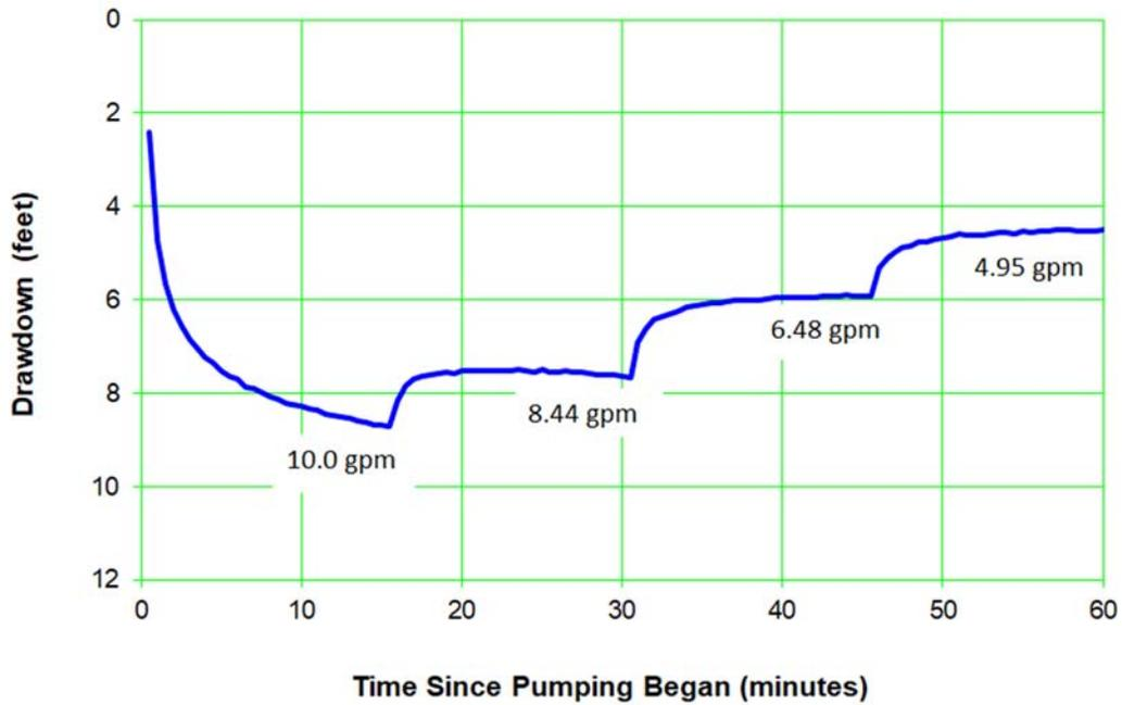
Figure A-3.1-1 Well R-7 screen 3 step-drawdown test response after jetting
