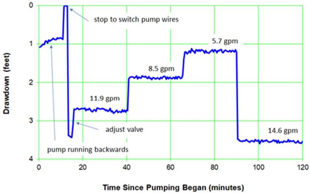
Figure A-5.0-1 Well R-9i screen 1 step-drawdown test response
