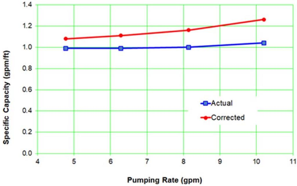
Figure A-3.0-2 Well R-7 screen 3 actual and corrected specific capacities
