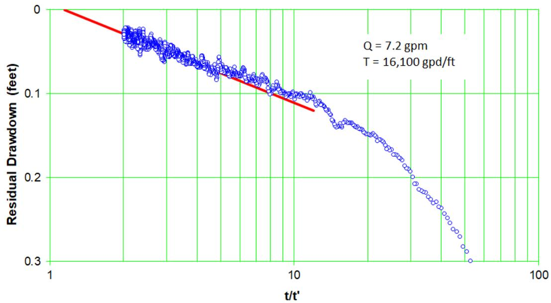
Figure C-8.3-7 Well R-7 screen 3 recovery – late data rolling average
