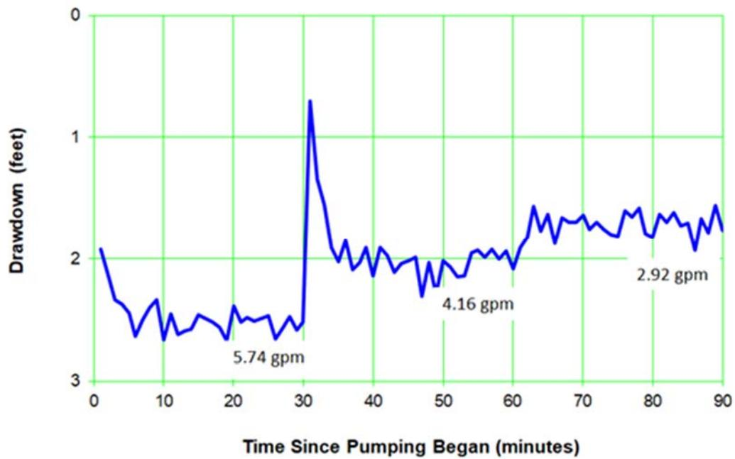
Figure A-6.0-3 Well R-19 screen 4 initial step-drawdown test response
