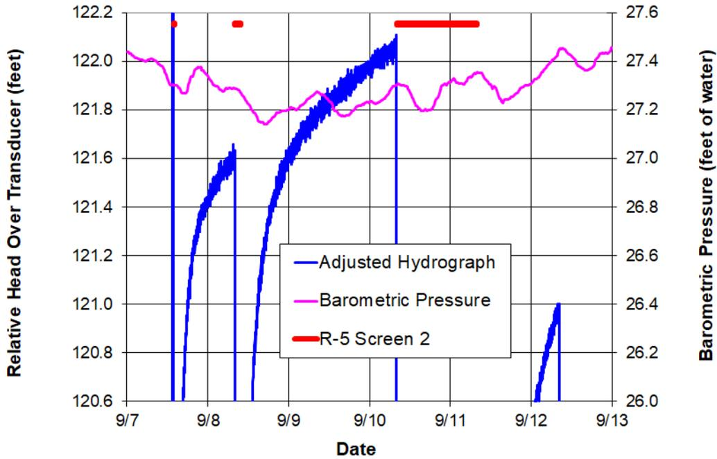
Figure C-7.2-1 Well R-5 screen 2 adjusted hydrograph
