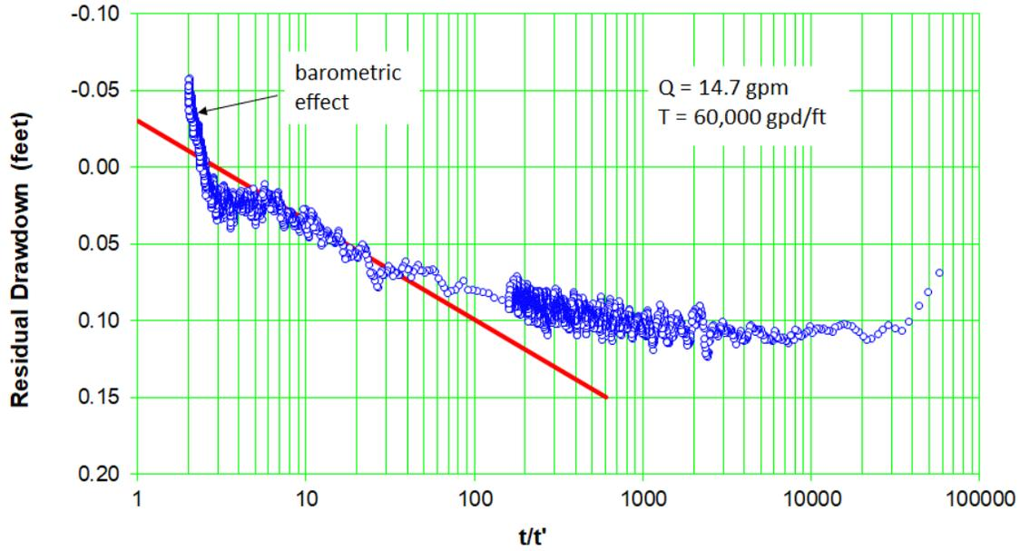
Figure C-10.3-17 Well R-9i screen 1 recovery – rolling average
