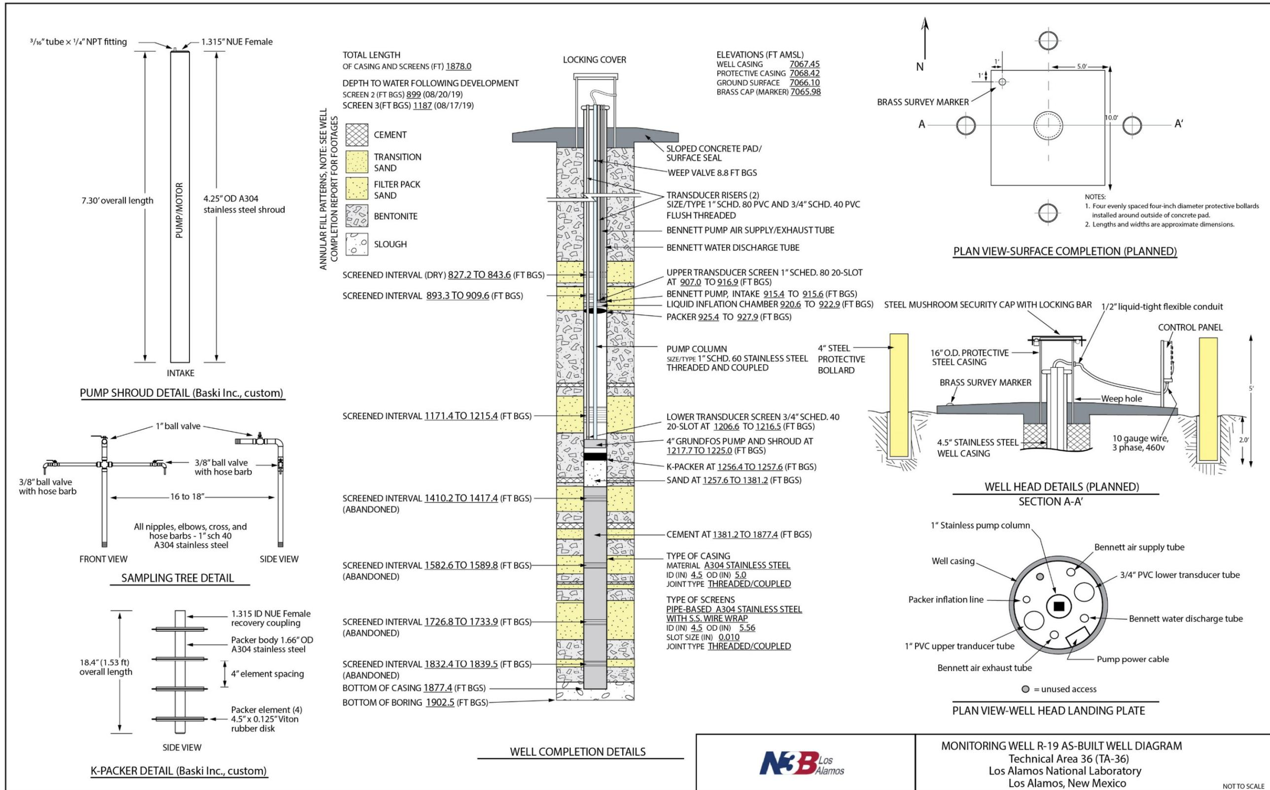
Figure 2.5-1 Monitoring well R-19 as-built construction diagram post-Westbay conversion
