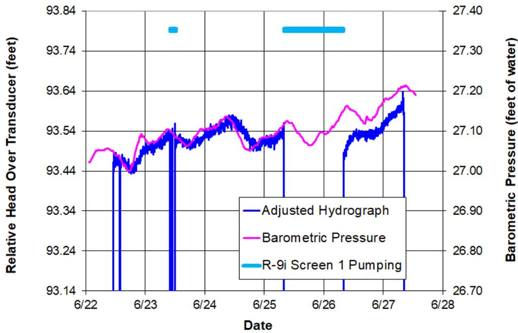
Figure C-10.2-2 Well R-9i screen 1 rolling average hydrograph and 45% barometric efficiency correction
