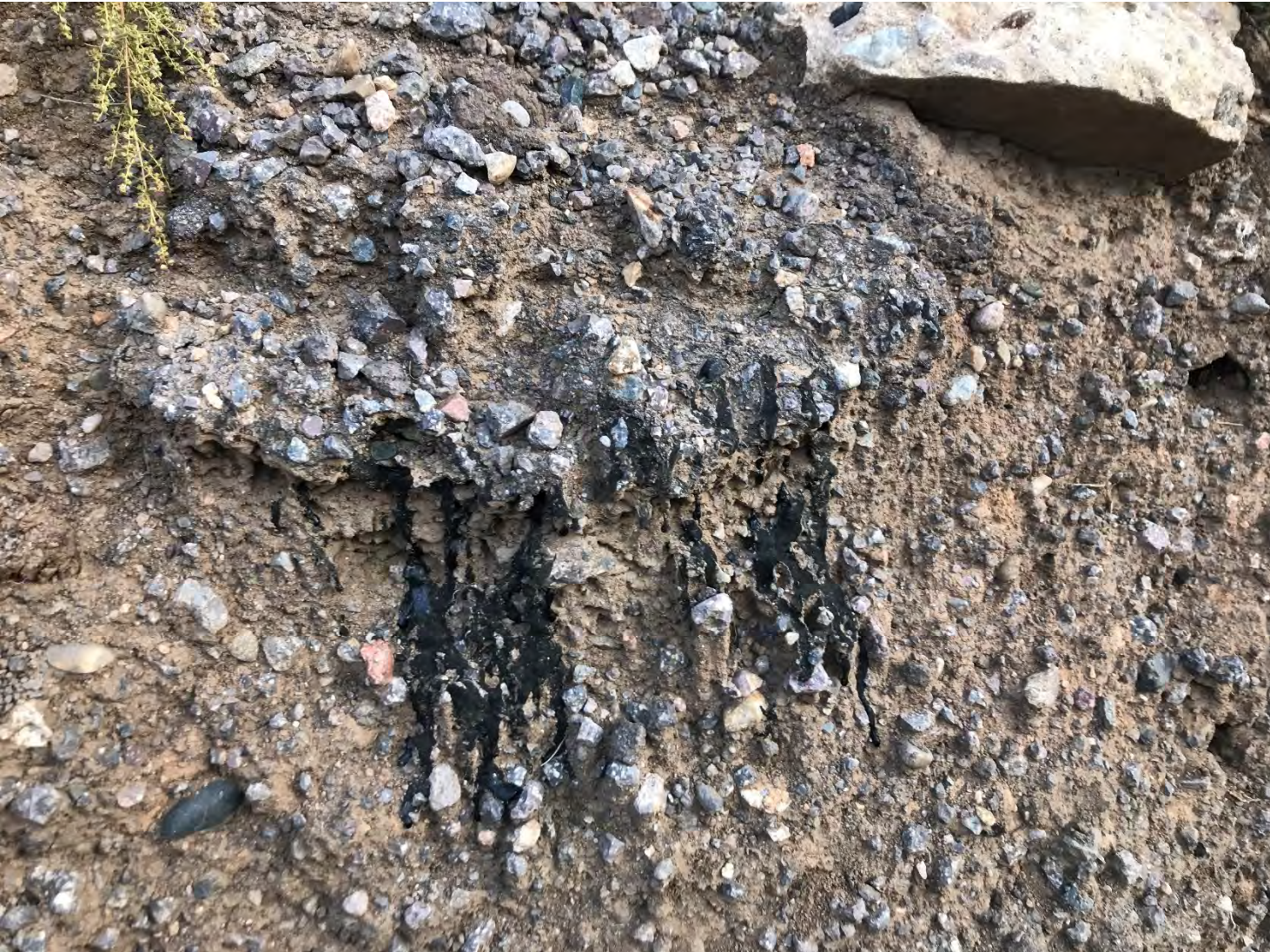
Figure 4.2-2 Example of tar and asphalt in the banks of the drainage channel. The visual portion of the piece of asphalt is approximately 1 ft in height and width.
