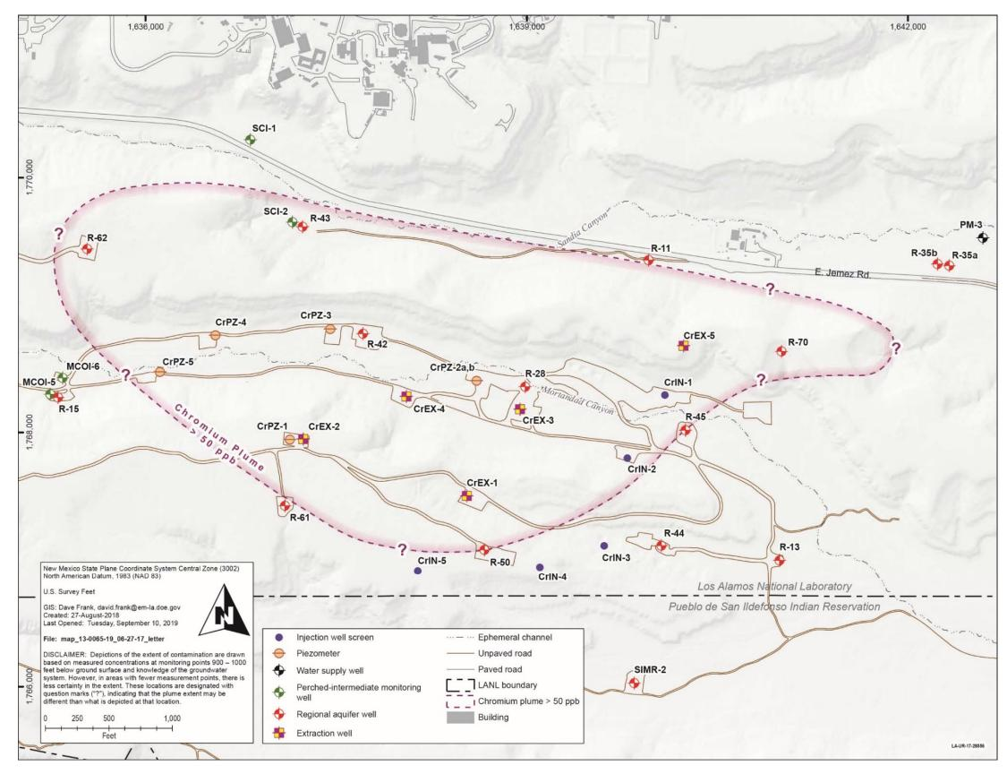
Note: Locations of monitoring wells, piezometers, extraction wells, and injection wells are also shown.
