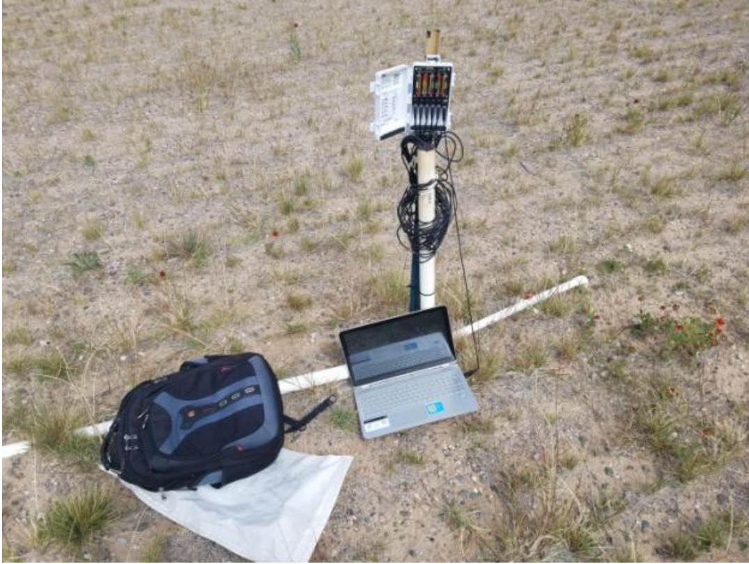
Picture 6. Water Balance Monitoring Nest - South Slope of Landfill
