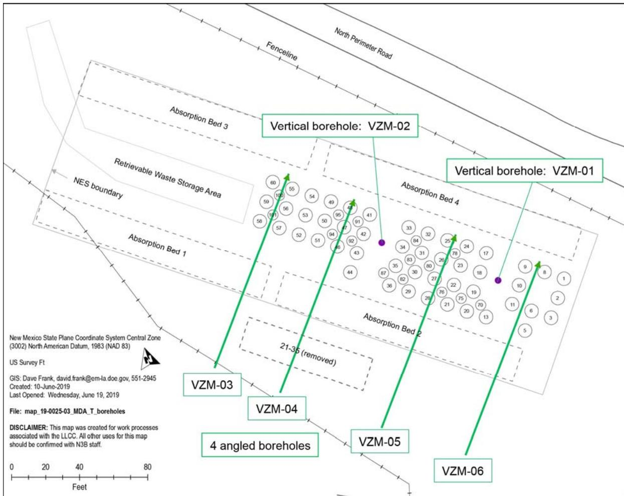
Figure 3.2-1 Locations of proposed vertical and angled boreholes at MDA T
