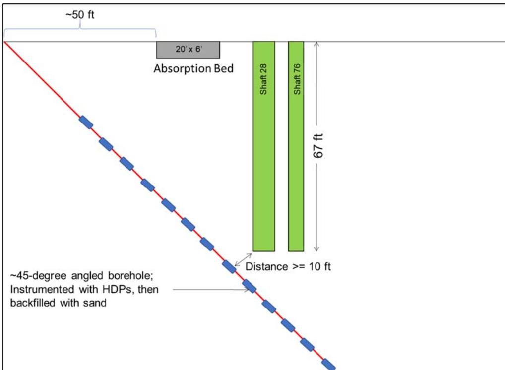
Figure 3.2-3 Cross-section schematic diagram of angled boreholes under shaft field
