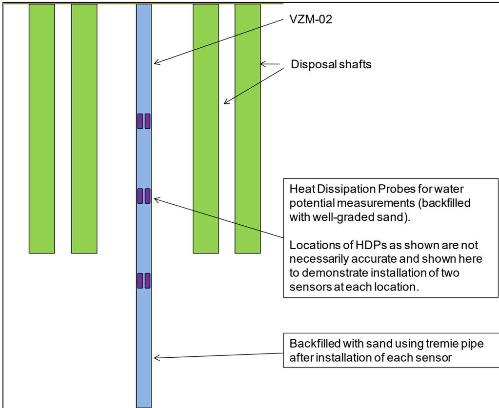
Figure 3.2-2 Cross-section schematic diagram of vertical boreholes in shaft field
